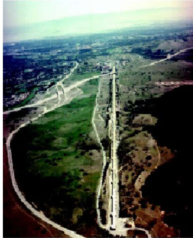
SLAC, two mile long, 50 GeV linear accelerator, most powerful electron accelerator in world
