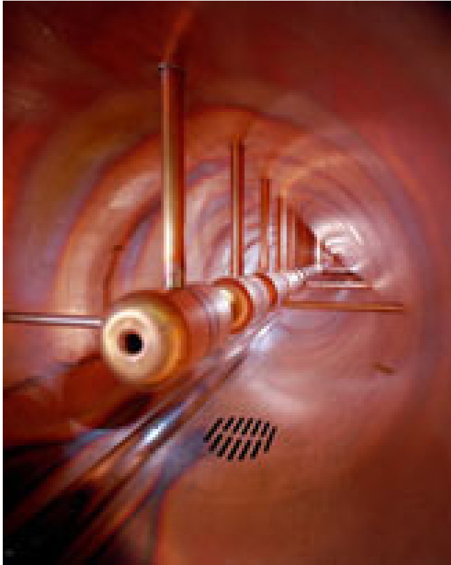
FNAL second stage linear accelerator (400 MeV)
